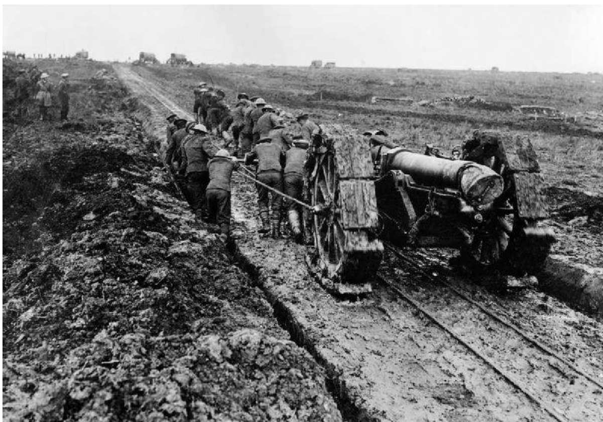
A 6-inch 26 cwt howitzer being manhandled through the mud during the Battle of the Somme 1916. The devices round the wheels to stop sinking were called girdles. ©IWM (Q1490)
